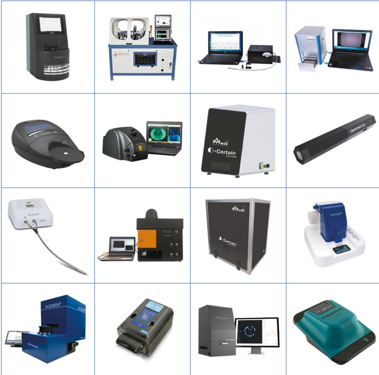
**Figure 3:** As of July 2019, the Assure Program had tested 16 diamond verification instruments. From left to right, these are: (top row) AMS2, ASDI, DiamondDect 3 and DiamondDect 5; (second row) DiamondSure, DiamondView, G-Certain and GemPen; (third row) GIA iD100, GV5000, J-Certain and Leo; (bottom row) M-Screen+, Sherlock Holmes, SYNTHdetect and Synthetic Diamond Screener II. These photos were supplied to the Assure Program by the instrument manufacturers.
